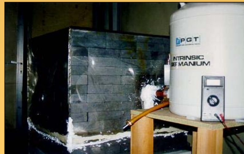
AMBAR for measuring radioactive contaminants in materials intended for low-background experiments
