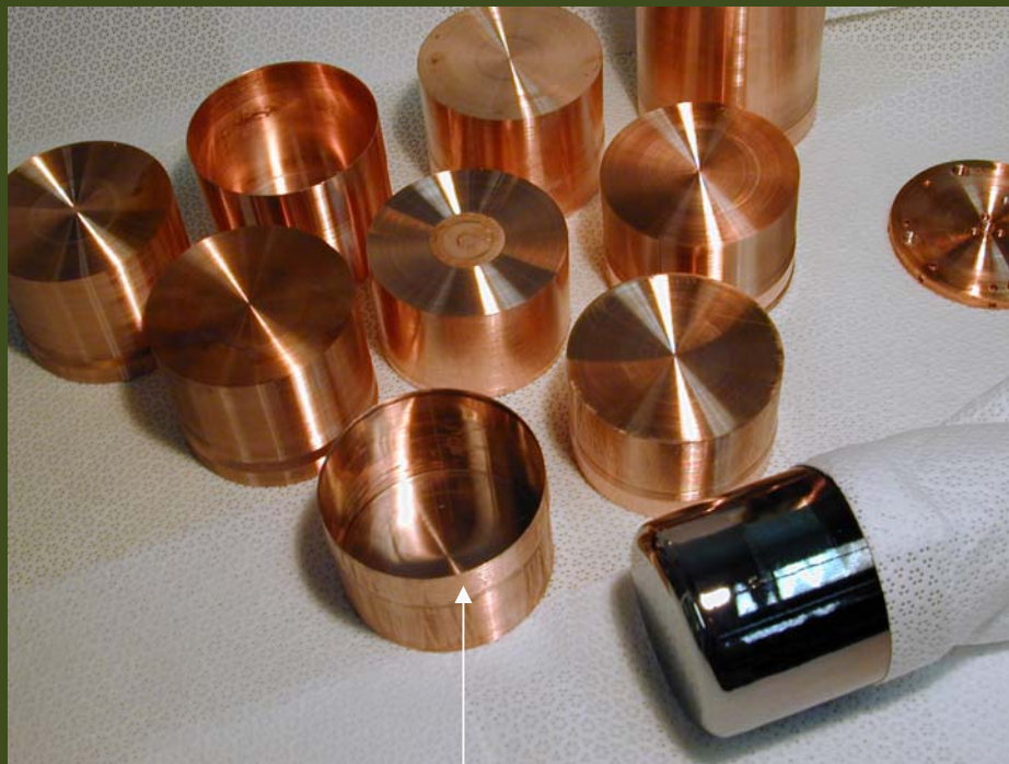
Electroformed cups shown have wall thickness of only 250 \mu m!
