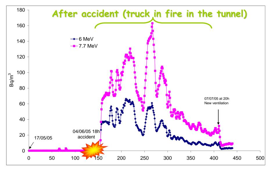
After the accident in the tunnel, ventilation and compressor went off
