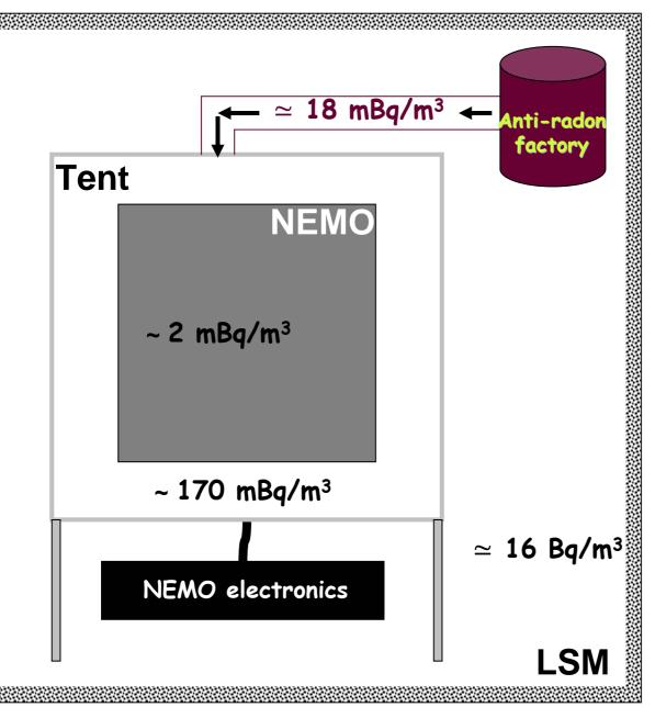
The difference between the activity injected and measured inside the tent due to:  $\Rightarrow$  air leaks in the tent  $\Rightarrow$  degassing of the NEMO electronics
